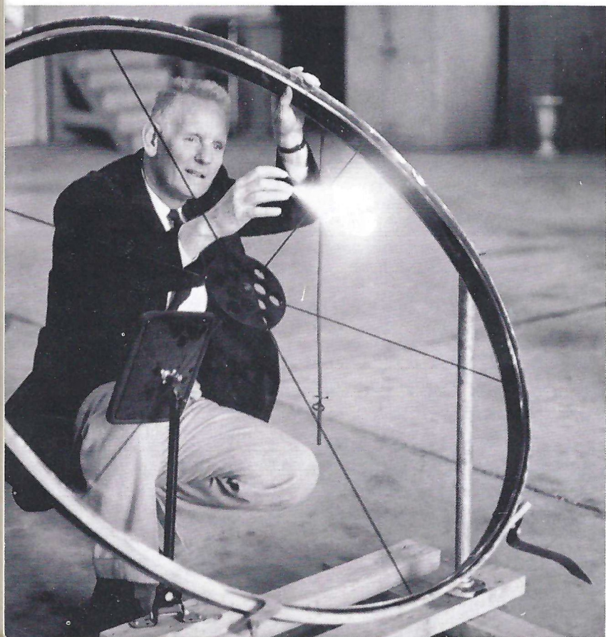
Dr. David T. Williams of the Department of Aerospace Engineering is working with plastic sheets to develop a reflecting surface which can be used for very large and very lightweight space mirrors in orbiting telescopes. Dr. Williams believes that such a telescope could make possible better pictures of the moon than can now be obtained.
